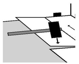
Click the second and remaining rows together rotating the boards horizontally at an angle of 20–30 Degrees. Gently tap the end joints into place using your rubber mallet. Ensure joints are staggered by at least 15cm.
