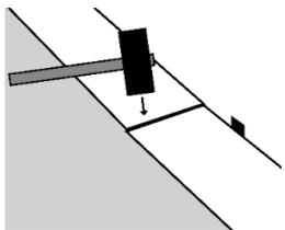
Use a soft rubber hammer to ensure the drop lock profile is properly engaged prior to installing the next plank.
