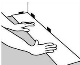
Install the first plank with spacers packed between the plank and the wall. Ensure the expansion gap is 12-15mm. **More expansion gap may be necessary in areas of high humidity. For example, Northern Queensland.**
