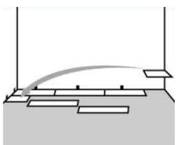
The offcut from the first row can be used as the first piece of flooring for the next row. Please ensure the 12 - 15mm gap is maintained throughout (**larger gaps in areas of high humidity**) the installation and ensure that the stagger between rows is at least 15cm.
