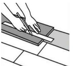
Make sure that the width of the last row is at least 5cm, and ensure that the gap around the perimeter of the floor remains at 12 – 15mm (**larger gaps in areas of high humidity**).
