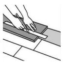
Make sure that the width of the last row is at least 5cm, and ensure that the gap around the perimeter of the floor remains at 10 - 15mm.
